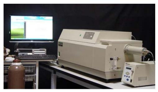
The J-810 offers hardware and software features to save time and deliver even better results. Instrument control and data processing are handled by user-friendly Spectra Manager for Windows PC platform. Increased Performance of the J-810's optical bench, with dual prism optics, and the 150-watt air cooled lamp housing provide remarkable stability and low maintenance cost.
